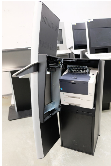
HERA 19" opened with A4-printer
